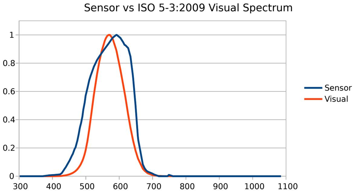
Fig. 8.4: Spectral response of the light sensor
