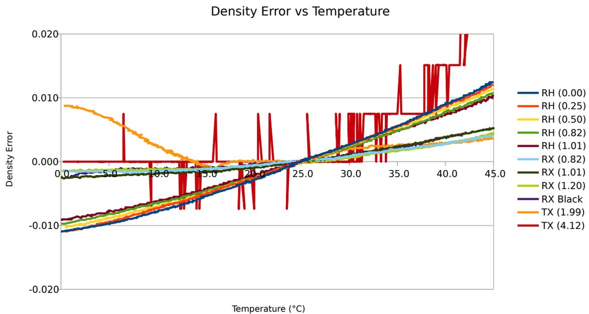
Fig. 8.5: Temperature sensitivity of density readings
