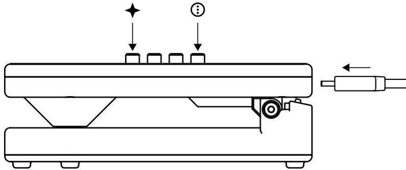
Fig. 6.1: Starting the bootloader
